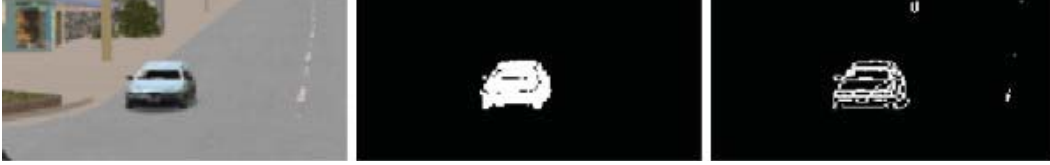
Figure 2: Detection matrix D for the GMM and the Level Lines algorithms.(left) Capture (center) GMM detection (right) LL detection
